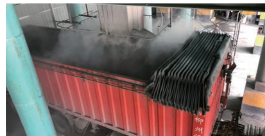
Dry fog dust fall at aggregates storage feed opening, Hongshuihe Cement
